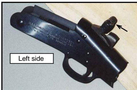
This side of the frame has the "splined" pin heads and in these instructions I'll refer to it as the **LEFT** side of the frame. Before you go further, you must remove the hammer extension with a allen wrench.
