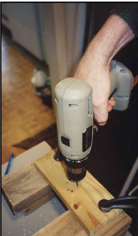
Drill the board using the impressions of the pins like center punch marks. Use the next size up drill bit from the pin size - for the large pins (3/16) I used a 7/32 bit, for the small one at the front of the triggerguard (3/32) I used a 7/64.
