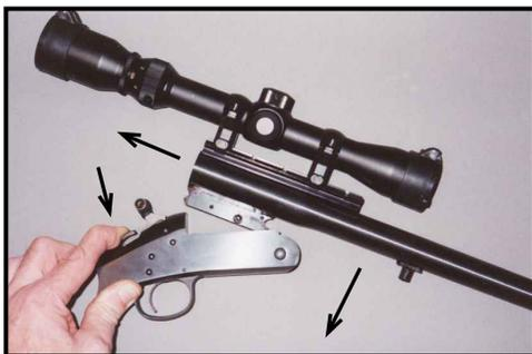
Depress the barrel catch release lever, then rotate the barrel down. While barrel is rotated down, lift barrel off to the rear and up. The side of the frame shown in the photo to the right I'll refer to as the **RIGHT** side in these instructions.
