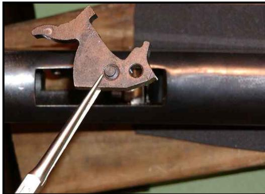
Now drive that pin completely out and again use your needle-nose pliers to wiggle the hammer out the bottom of the frame.
