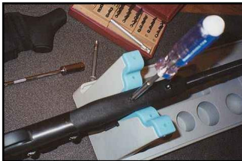
When you have removed the fore-end screw, pull fore-end down and away from frame.
