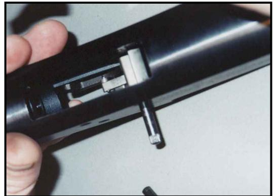
That only leaves the started pin that retains the barrel catch and lifter assembly in place. You want to remove the assembly as a unit, so have your slave pin handy.
