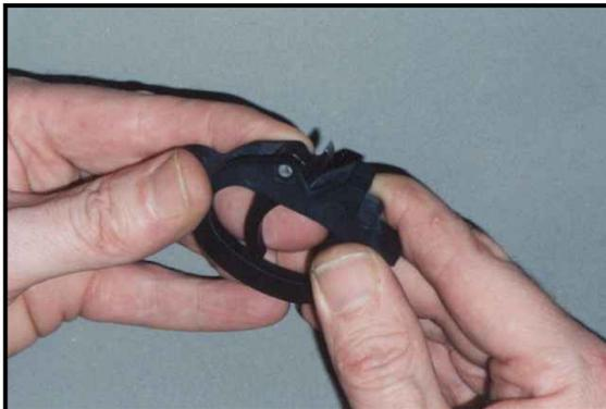
Note that the slave pin is flush with the sides of the guard at the trigger pivot point (not sticking out), but will hold the trigger in place as you reassemble the gun. It is also useful in holding the lifter, barrel catch, and spring assembly together when disassembling and assembling.
